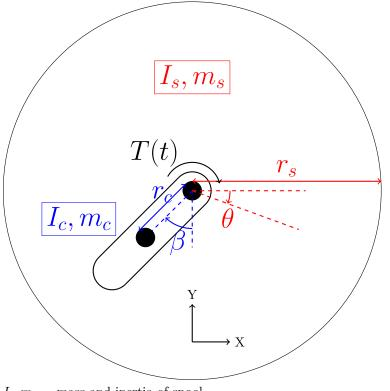
$$\begin{split} I_s, m_s &= \text{mass and inertia of spool} \\ I_c, m_c &= \text{mass and inertia of counterweight} \\ r_c &= \text{radius from COM spool to COM counterweight} \\ r_s &= \text{radius from COM spool to outer edge} \\ \theta &= \text{angle of spool (CW+)} \\ \beta &= \text{angle of counterweight (CW+)} \end{split}$$
